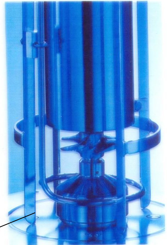
Plant Cell Fermenter
