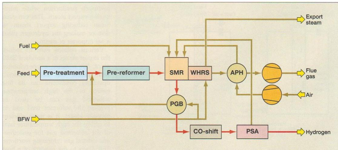
Figure 1 Typical H<sub>2</sub> SMR configuration: WHRS – waste heat recovery section, APH – air preheat, PGB – process gas boiler, PSA – pressure swing adsorption, BFW – boiler feed water
