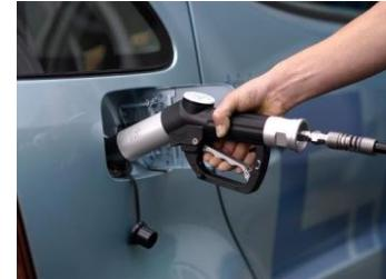
Fuel cell vehicles are limited in availability and depend in part on access to **refueling stations** for hydrogen.
