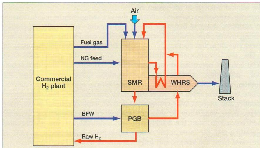
Figure 6 Block flow diagram of the multipurpose SMR demonstration plant;
