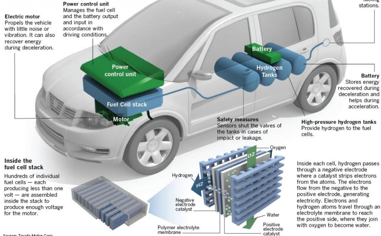
Inside each cell, hydrogen passes through a negative electrode where a catalyst strips electrons from the atoms. The electrons flow from the negative to the positive electrode, generating electricity. Electrons and hydrogen atoms travel through an electrolyte membrane to reach the positive side, where they join with oxygen to become water.
