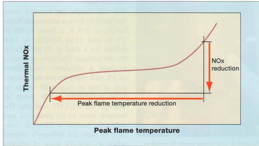
Figure 3 Peak flame temperature versus thermal NOx production
