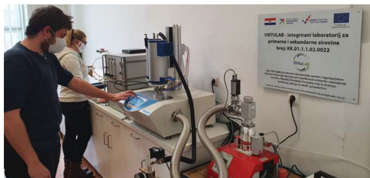
Figure 2. Differential scanning calorimeter with two furnaces and a total working range of -150 to 1600 °C, model HDSX-PT 1600, Linseis GmbH, Germany, installed in one of the laboratories of the Department for Inorganic Chemical Technology and Nonmetals.
