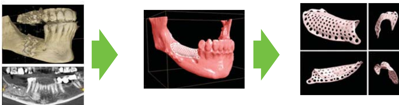
Figure 1. A schematic illustration of an individualized implant production – a biodegradable 3D printed mesh according to CT scans of the patient's jaw.
