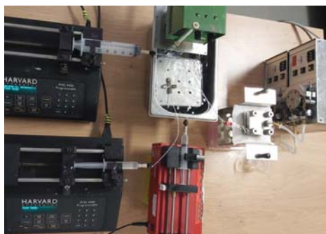
Figure 2. Scheme of an integrated microsystem for the production and purification of biodiesel by ultrafiltration.
