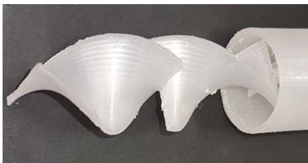
Figure 2. 3D printed model of a static mixer for chemical reaction intensification.
