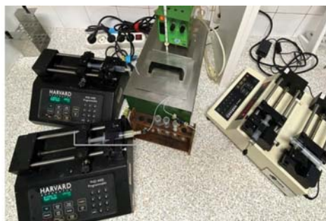
Figure 3. Scheme of an integrated microsystem for the production and purification of biodiesel by extraction with eutectic solvents.
