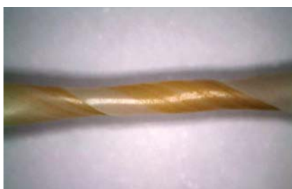
Figure 4. Bending of modified PEDOT conductive polymer.
