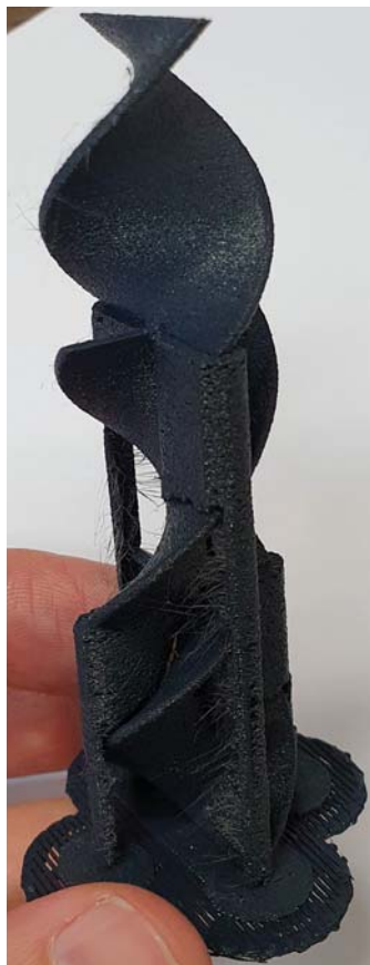
Figure 3. 3D printed model of a static mixer for chemical reaction intensification. This static mixer is made of nanocomposite based on PETG, TiO 2 and CNT.
