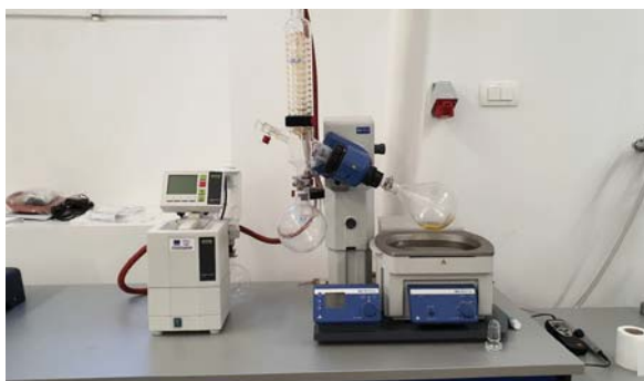
Figure 2. The solvent preparation system: vacuum pump is connected to a rotary evaporator. It's used to prepare deep eutectic solvents for purifying raw materials and crude biodiesel.
