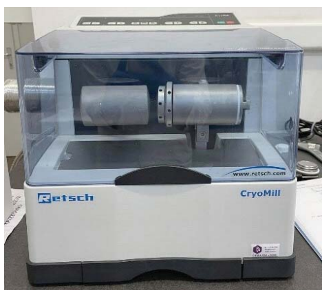
Figure 1. Cryogenic ball mill for the preparation of unaged and aged plastic samples.
