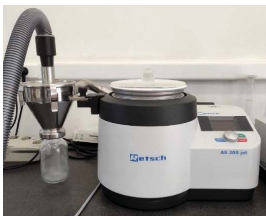
Figure 2. Laboratory air jet sieve for separating size fractions of MPs.
