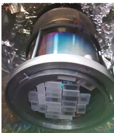
Figure 2. Samples on the carrier, prepared for processing and placed in the Hybrid Plasmionique reactor.
