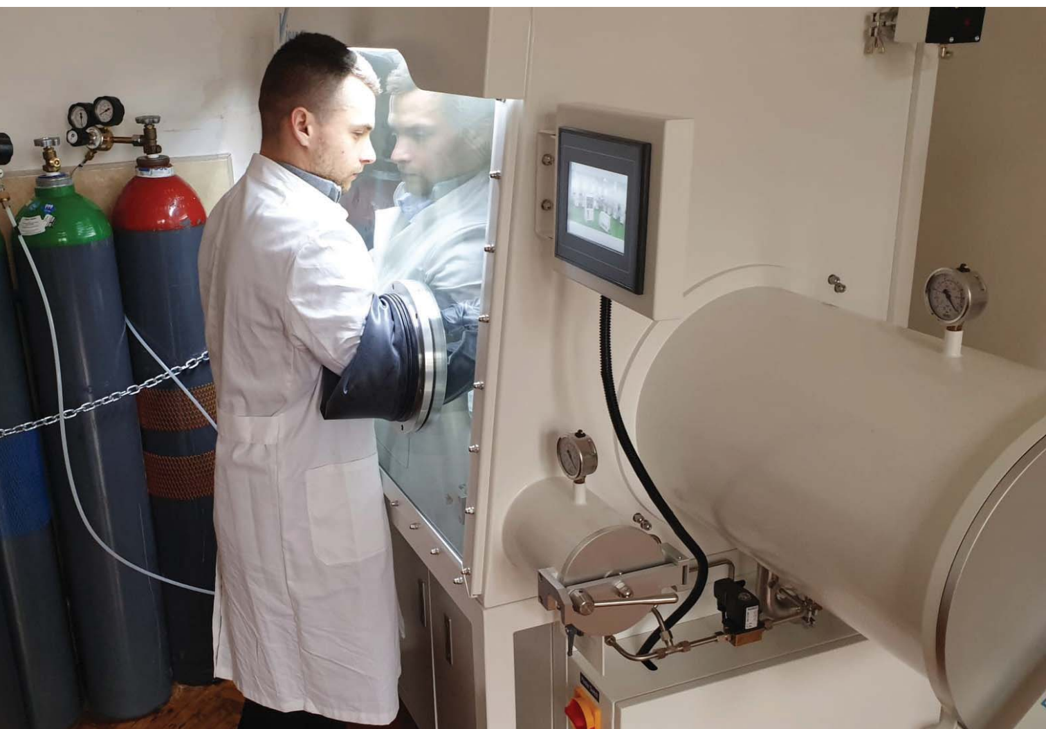
Figure 1. Grgur Mihalinec during the assembly of a battery cell in the glove box.
