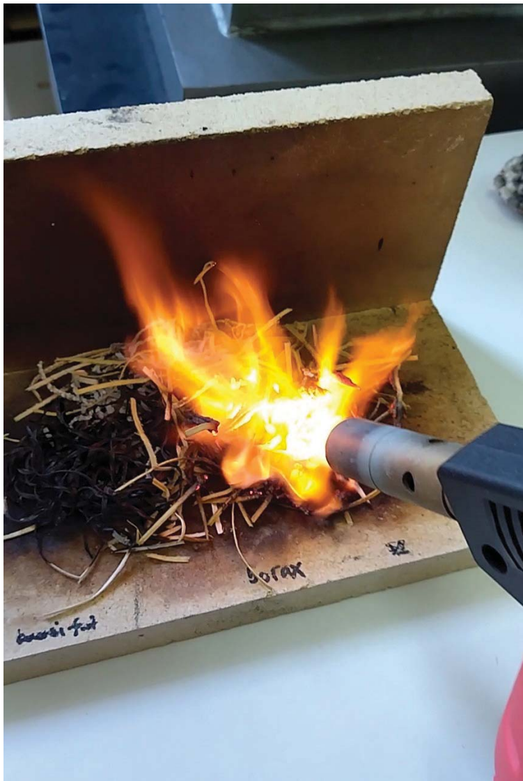
Figure 3. Laboratory test of the fire-retardant additive for wood wool.
