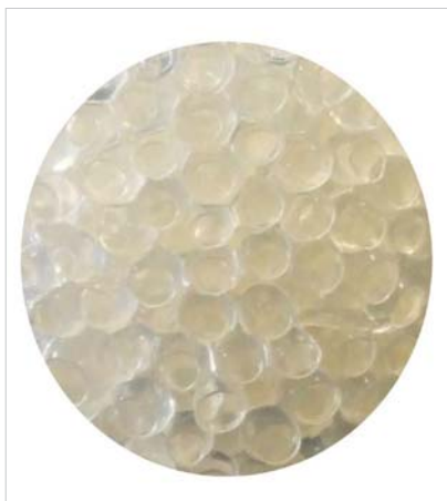
Figure 1. E. coli cells containing halohydrin dehalogenase immobilized in calcium alginate.
